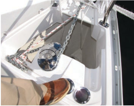
ABOVE: Double bow rollers, Maxwell RC10 windlass and a deep locker should ensure stress-free anchoring with the Catalina 355.
